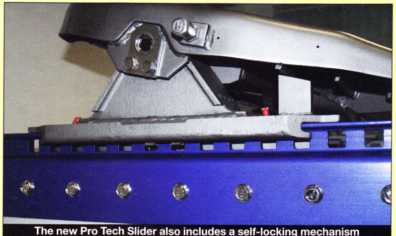
The new Pro Tech Slider also includes a self-locking mechanism
